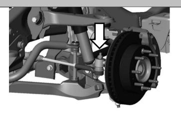
Unscrew inner tie rod from center link by unscrewing inner ball joint.
