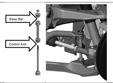
Repeat the above steps for installing the other tie rod and sway bar end link on the opposite side of the vehicle.
