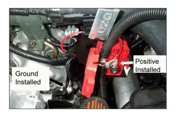
2. On LMM (2007-2010) trucks, connect the positive to the small stud on the driver side battery terminal, and connect the ground to either the battery negative or to a body ground.
