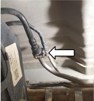
Locate the factory fuel line disconnect at the top of the fuel cooler, directly ahead of the fuel tank
