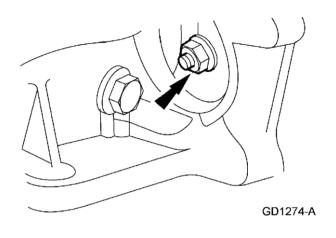
**NOTE:** Do not over-torque these fasteners!
