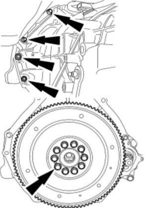
Install BD Diesel flexplate onto the crankshaft, followed by the washer.
