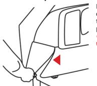
Remove the panel on the side of the dashboard to provide access to route the OBDII/HDMI cable from the OBDII port up to the top of the dash.
