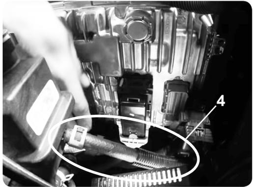
**STEP 5** - Disconnect the center, small black connector by sliding and pressing in the green tab, and then open the clamp until it disconnects.
