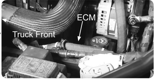
**STEP 2** - Remove the small blue connector (closest to the front) from the ECM by holding in the tab and carefully opening the clamp until it disconnects.
