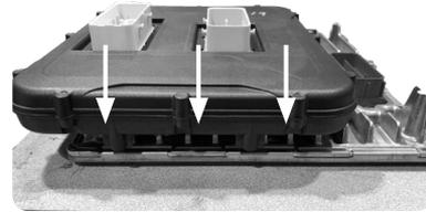
**STEP 4** - Install the second bracket piece (b) to the Assembly by sliding it into place near the bottom of the Pulsar module, then insert the provided screws and tighten until snug.
