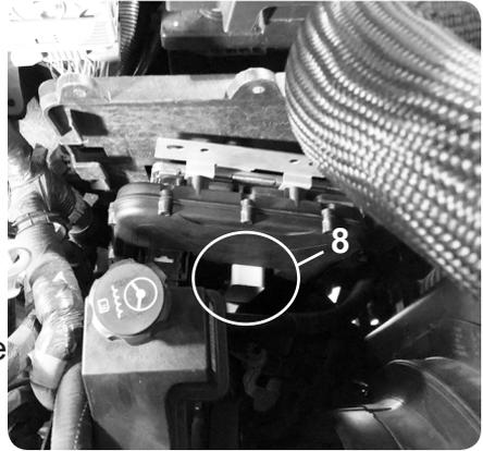
**STEP 9** - Lift Assembly up to the stock bracket, then carefully insert the ECM into the stock bracket by sliding down and back.
