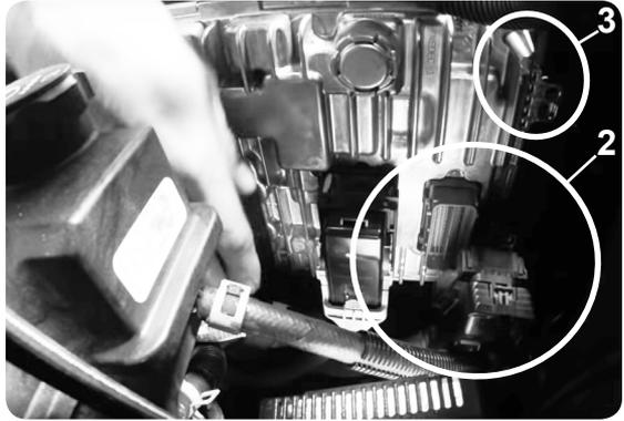
**STEP 3** - Depending on truck year, remove the plastic push rivet (2017), or remove the 10mm bolt (2018-2019) holding the ECM to the bracket, located on the top front corner of the ECM.
