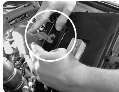
**STEP 6** - Take Assembly back to the engine and reconnect the large black connector harness, then carefully close the clamp once connector is completely set in place. Slide the green tab back into place to lock.
