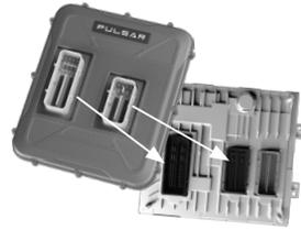
**STEP 2** - Carefully, yet firmly push the Pulsar module down onto the ECM. Ensure the device is pushed directly down and not at an angle. Push until the Pulsar is flat against the ECM.
