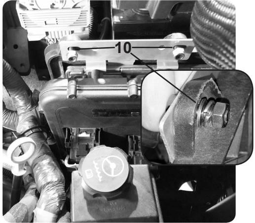
**STEP 11** - Using a 10mm hand wrench with a socket wrench, tighten the nut and bolts until snug.
